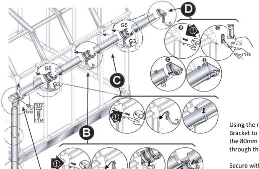
Attach a Fascia Bracket to the R1 Round profile, opposite to the end where the downpipe will be positioned, using a self tapping screw.
