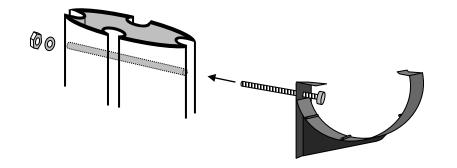
Remove both the inner and outer pins from the top holes in the E1Oval and R1 Round profiles that make up the walls of your greenhouse.
