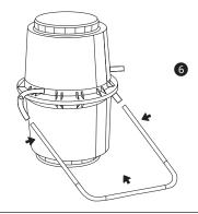
Fit one leg set to elbows by pressing "U" shape together sufficiently to allow entry to elbows.
