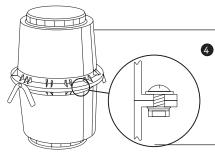
Assemble drum by placing second half on top of first half making sure to locate bearing grooves. Join drum halves together using drum joining screws (J). Fit 16 screws with washers in holes before adding and tightening nuts.
