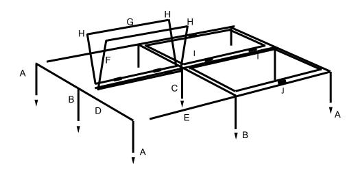
4. Once the main frame and lids are assembled, lock the lid hinge joints in place against the central length tube "E" using the self-tapping grub screws. Set each hinge at approximately 45\* to each other.
