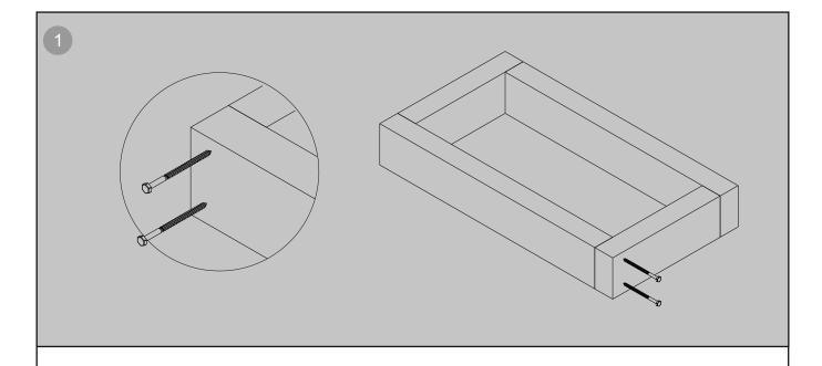
Place the sleepers on the ground placing each sleeper as shown to create a rectangle 1300 x 700mm.
