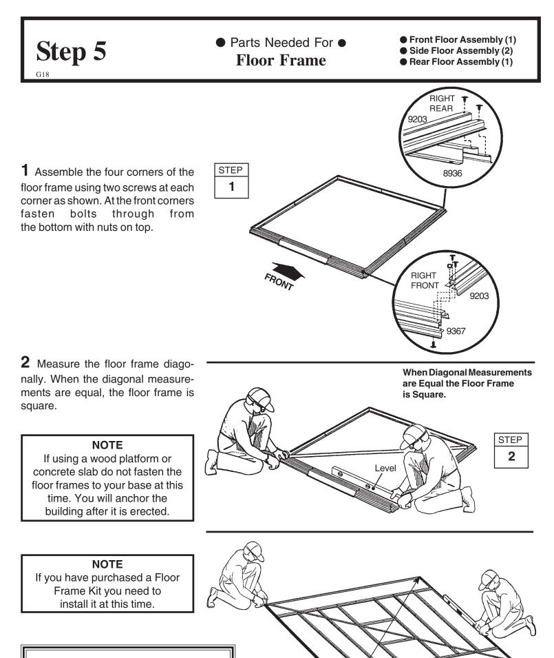
The floor frame *must be square* and *level* or holes will not align.
