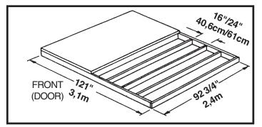
Note: Platform/Slab will extend 9/16" (1,4cm) beyond floor frame on all four sides. Seal this 9/16" of wood with a roofing cement (not included), or bevel this 9/16" of concrete when pouring, for good water drainage.
