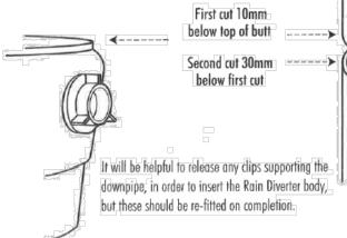
Remember, If correctly fitted the Rain Diverter will always fill the butt to the level of the diverter connector. Should a fitting error occur correct as follows:
