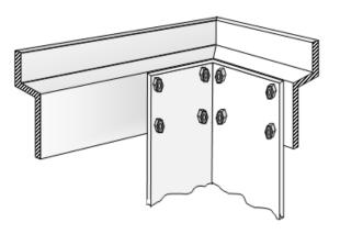
Attach the four top frame "Z" sections to the outside of the four corner legs finger tight only.
