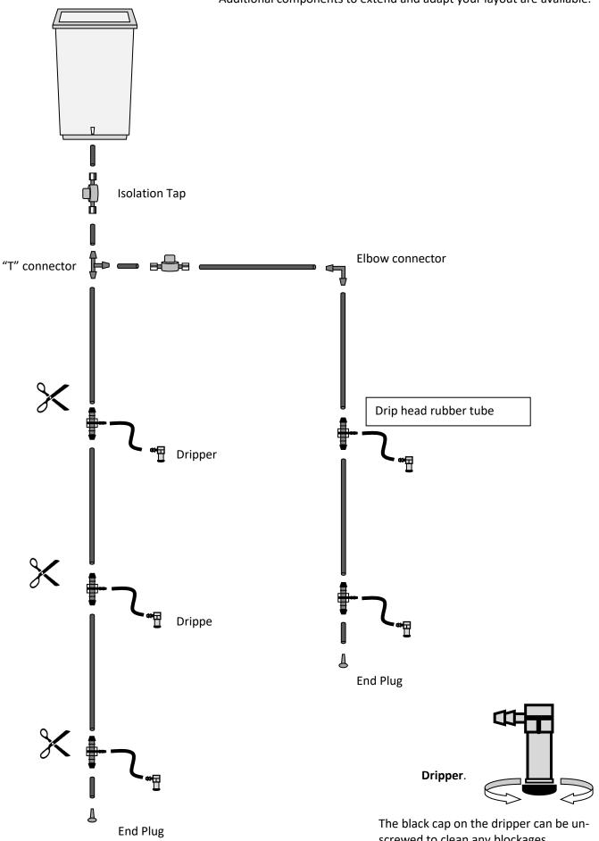
This diagram gives you an idea where each of the components can be placed. Additional components to extend and adapt your layout are available.
