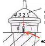
Turn the top of the dripper so that the desired setting lines up with the exit hole for the water.
