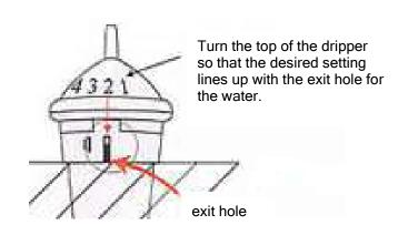
Each dripper can water an area up to 10" / 25cm in diameter. Depending on the area being watered will affect how many drippers you will need to use. Please note - when the drippers are first used the water may run faster but the drip rate will settle down to the correct speed after about 7 days.
