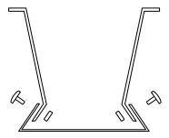
5. Lower the assembled plates into the frame and bolt in position. Once all the bolts are in square up and tighten fully.
