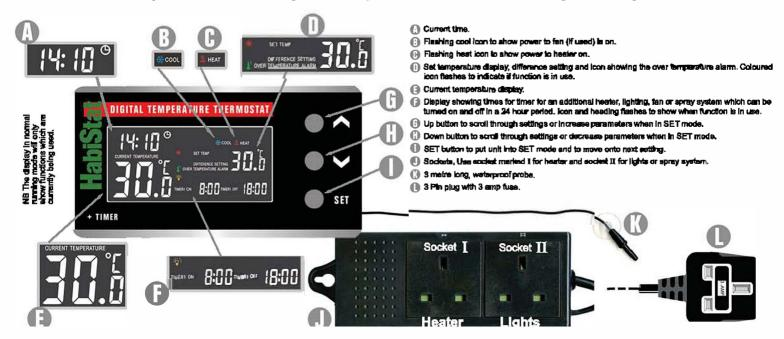
**SETTINGS**. Press the **SET** button and hold for 3 seconds. This puts the unit into SET mode. Use the **A V** buttons to change parameters (hold button down for rapid change) and then press **SET** to save and move onto the next setting. The order is shown below. Elements **highlighted** indicates flashing display.
