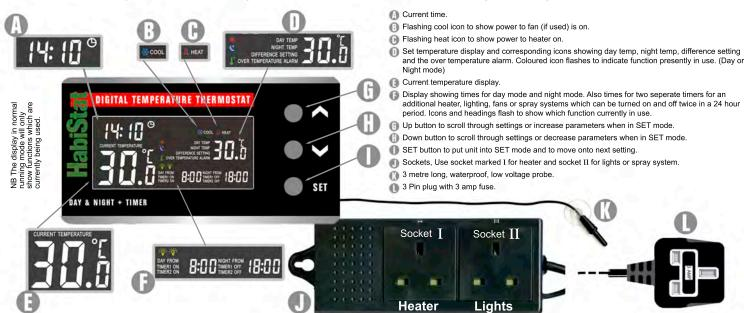
Quick check of settings. Settings can be quickly checked without going into the setting routine. Simply scroll up or down with the Λ V arrows. Functions will scroll through and will flash indicating current settings of those functions flashing. You cannot alter these settings in this manner and the normal display will resume if untouched for 5 seconds.
