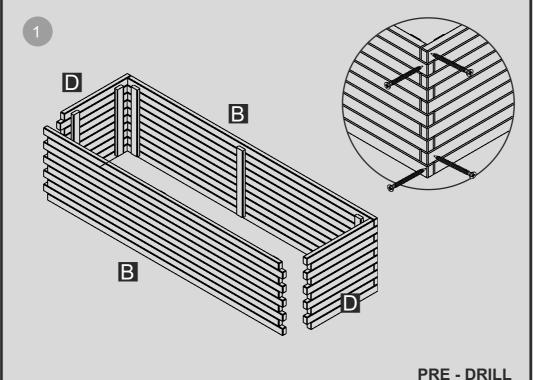
Slot the side and end sections together.
