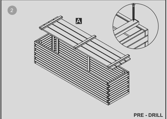
Place the base on top so that the bearers are sat on the side sections.
