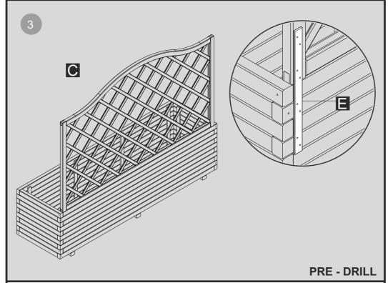
Fix a steel plate to each end of the trellis back using four of the holes and 25mm screws for each plate.
