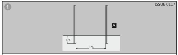
Position the posts in a square formation as shown and sink 375mm into the ground.
