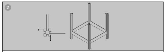
Slot the first row of boards into the framing. Secure 3 of the boards using the 50mm screws, 2 at each end of each board. The one board you do not secure will be your access to the compost so position it in an accessible orientation.
