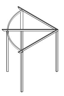
Place Rafter 4 so that the notch overlaps the join between the two arc rafters and sits on the un notched post central, between the other rafters.
