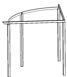
Slot the Rafter 1 and 7 onto the ends of the arc rafters as shown. Make sure that they in line with each other and the un notched post.
