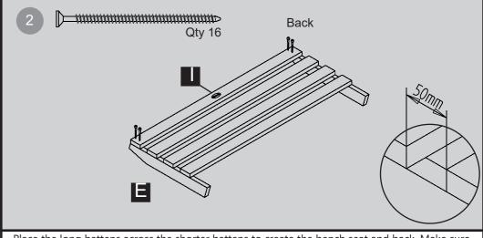
Place the long battens across the shorter battens to create the bench seat and back. Make sure that the battens for the bench are spaced 50mm apart. Fix each in place using 2x60mm screws for
