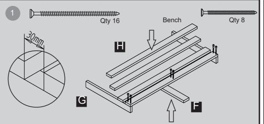
Make sure that the battens for the bench are spaced 30mm apart. Fix each in place using 2x60mm screws for each end.
