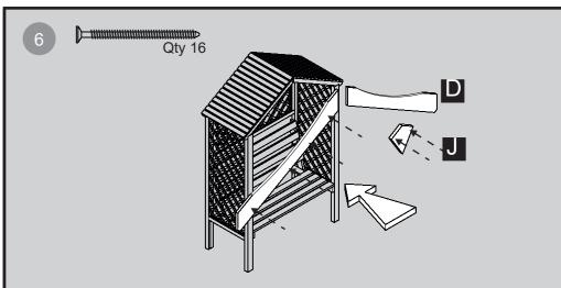
Place the barge boards to the roof so that the bottom of the curve is in line with the top of the roof and they meet at the apex. Fix each in place using 3x40mm screws, Place the finial over where the barge boards meet and secure each in place using 2x40mm screws.
