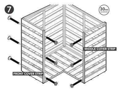
Secure the Front Cover Strip and Middle Cover Strip. Ensure the strips are flush to the bottom board on the panels.
