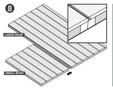
Tap the Small Roof into the Large Roof with a mallet. Ensure the battens are flush together when slotting together. If a mallet is not available, use a wide piece of wood to protect the product when hammering.
