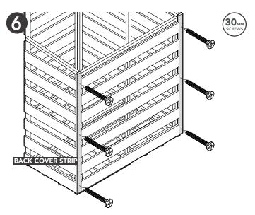
**Secure the Back Cover Strips.** Ensure the strips are flush to the bottom board on the panels.
