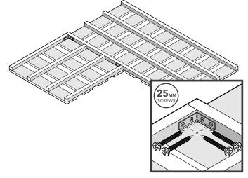
Turn the floors upside down. **Position and secure 2 x L-brackets** to the corners of the **Small Floor** as shown above to secure the floors together.
