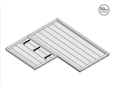
Once the roof panels have been slotted together, turn them upside down and **secure the roof panels together** as shown above.
