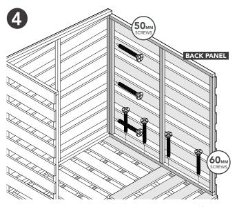
Attach the Back Panel to the side panel and floors as shown above. Use 60mm screws for the floor and 50mm screws for securing the panels together.
