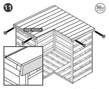
Attach the Side Fascias. Ensure the fascias are flush to the inside roof face as shown above. There will be a slight overhang from the Side Fascia's.
