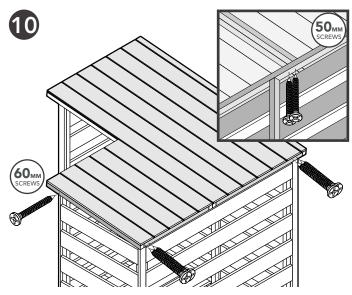
Secure the assmbled roof panels to the Cover strips, Back Panel and Right Side Panel as shown above. Screw through the top batten of the Back Panel into the roof battens that are resting on the Back Panel.
