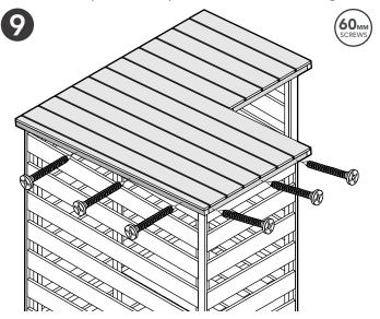
Position and attach the assembled roof panels to the panels. Ensure the roof is pushed up against the Left Side Panel and Front Panel to secure into place.
