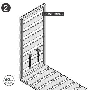
**Secure the Front Panel.** Screw into the bearers of the floor beneath. Ensure the panel is flush to the edges of the floor.
