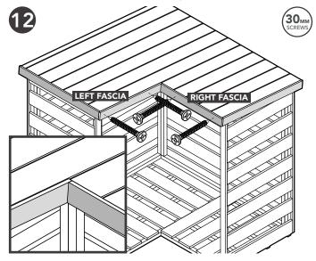
Attach the Left and Right Fascias to the roof panels as shown above. Ensure they are flush to the Side Fascias.
