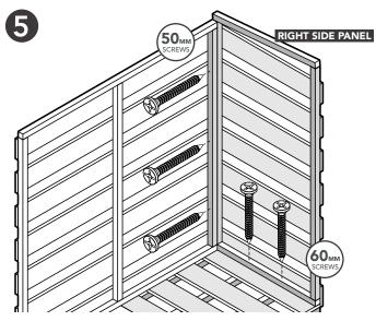
Attach the Right Side Panel to the Back Panel and Small Floor as shown above. Use 60mm screws for the floor and 50mm screws for securing the panels together.
