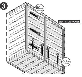
Attach the Left Side Panel to the Front Panel and Large Floor as shown above. Use 60mm screws for the floor and 50mm screws for securing the panels together.
