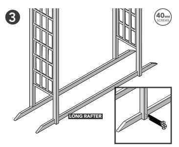
Position and secure the Long Rafters to the Posts. Ensure the Long Rafters are flush to the top of the Posts. Space out the arch to your desired width.
