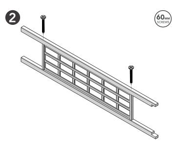
Position and secure another Post to the other side of the Trellis. Ensure the notched ends on the Posts are as shown above. Repeat the process for the other side.
