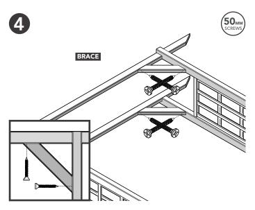
Position and secure the Braces to the Long Rafters and Posts, as shown above. Repeat on the other side.
