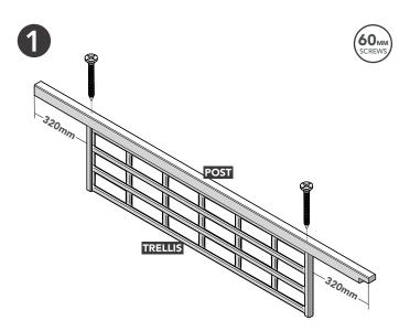
Position a Post on top of a Trellis, using the measurements provided. Screw from the outside into the top and bottom of the Trellis as shown above.
