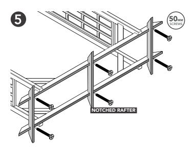
Position and secure 2 x Notched Rafters to the ends of the arch as shown above. Secure 1 x Notched Rafter in the centre of the Long Rafter. Ensure to space the Notched Rafters evenly.
