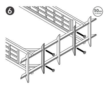
Position and secure the remaining Notched Rafters to the Long Rafters.
