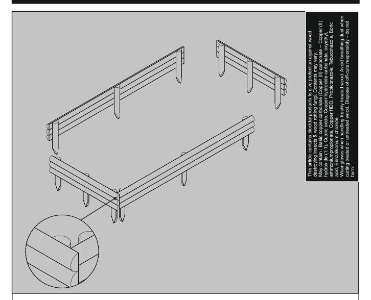
Place the log sections together as shown. Secure these in place using 2x50mm screws Position these in the top and the bottom logs.
