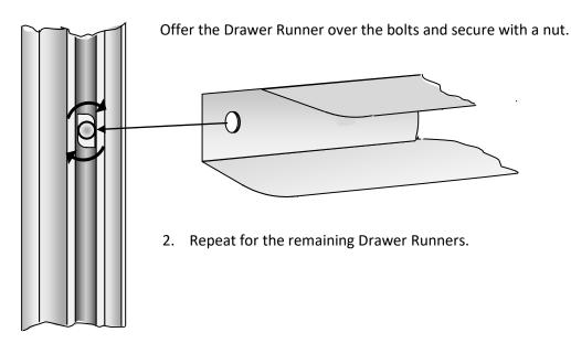
3. At the same level of each pair of Drawer Runners, insert a further two cropped bolts into the channel that will be at the back of the unit.
