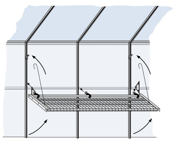
6. Position the two suspension wires through the mesh so that one end hooks under the front central shelf rail. The two wires then locate in the two brackets bolted into the glazing bars. Adjust the brackets as necessary so that the staging sits horizontal and tighten fully.
