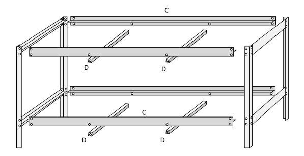
3. Bolt the four support bars to the lower part of the Length Horizontals.
