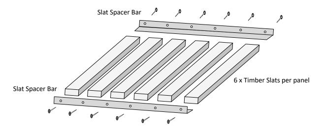
4. For the Timber Slatted option assemble each panel as shown above using the wood screws provided.
