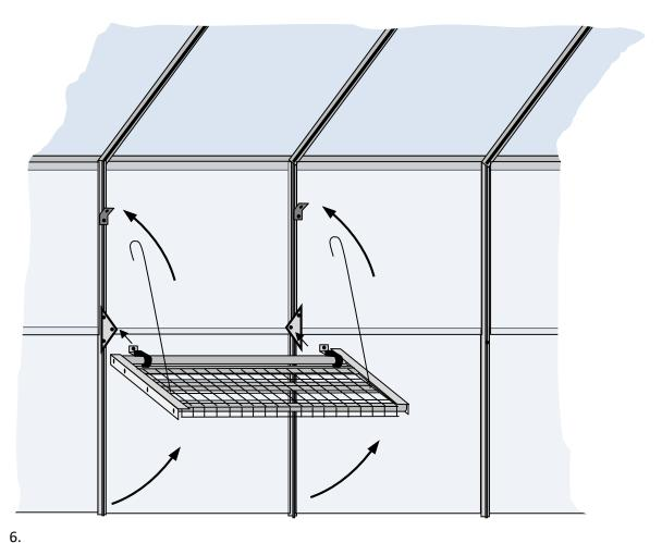
Position the two suspension wires through the mesh so that one end hooks under the front central shelf rail.
