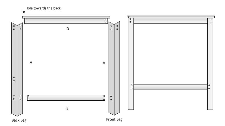
Join the two end sections together using the length "Z" sections making sure that the one with the additional hole at each end is to the back.
