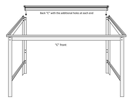
Attach the two Top Shelf Uprights to the outside of the top edge of the main frame.
