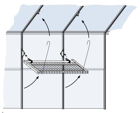
6. Position the two suspension wires through the mesh so that one end hooks under the front shelf rail.
