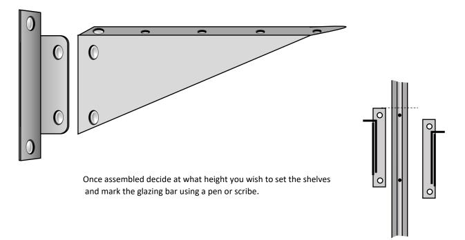
Insert two of the cropped bolts into the fixing bracket and offer up to the glazing bar of the greenhouse, level with your mark, and secure with two nuts.
