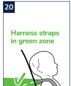
Harness straps in green zone The shoulder straps must be in the slots which are nearest to the child's shoulders but not more than 25mm below the child's shoulders
