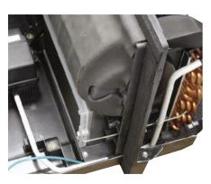
INTERNAL CONDENSATE REMOVAL (ICR)<sup>°</sup>
