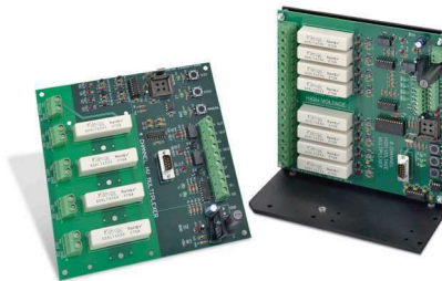
Multi-Channel High Voltage Switching Sequencer for up to 8 ultrasonic converter stacks
