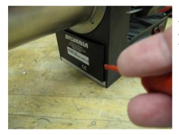
Using a flat head screwdriver remove the terminal cover from the base housing to expose the terminal strip where the blower terminals will land.
