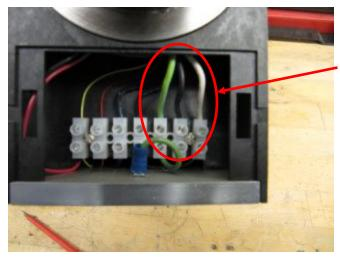
Photo shown is with our standard blower. The blower leads are the green (ground), black (hot), and white (neutral) on the right most top terminals. Simply wire to these same terminals using the leads from the external blower and the blower switch on the Skorpion unit will power the external blower. With this setup the heater coil cannot be energized without the blower being turned on first.
