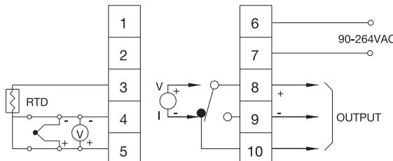
**NOTE:** Terminals 8, 9 and 10 are not used for Model TEC-900.
