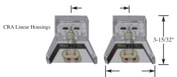
Minimum Spacing between Heaters in Array Assemblies ("D" Dim.) and CRA Linear Housings
