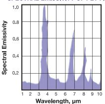
**WAVELENGTH CONTROL** – The very low heat transmission losses through the clear quartz material of the twin bore heaters allow Tempco's engineers to carefully design the peak emitted wavelength of these heaters to match the peak absorption wavelength for a given material or application. By modifying the temperature of the E-mitter, its peak emitted wavelength will change according to Wien's displacement law (see page 7-101). All E-
