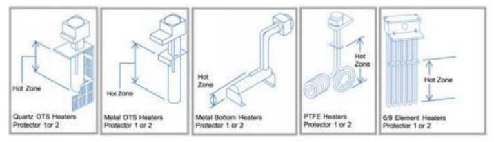
Figure 1: Typical Electric Immersion Heaters and their A vailable Over-temperature Protectors
