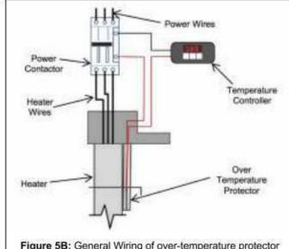
Figure 5B: General Wiring of over-temperature protector wired in series with temperature controller output to operate a power contactor.
