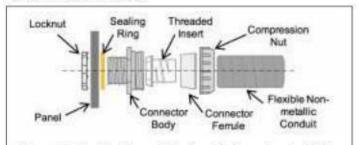
Figure 3B: Flexible Non-metallic Conduit Connector Installation
