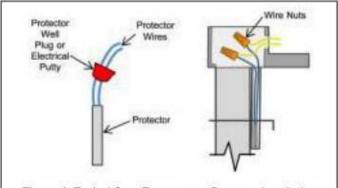
Figure 4: Typical Over-Temperature Protector Installation
