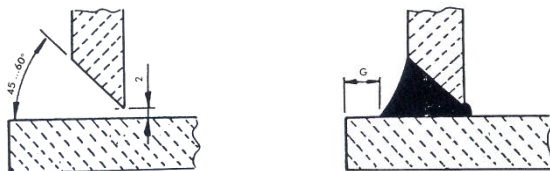
Joint to be welded
