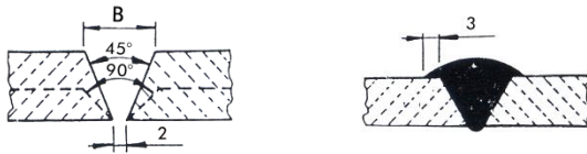
Separate joint to be welded
