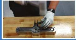
The Nextflex staking tool is a key component to seat the heater properly, improve heat transfer and maximize heater life. Strike hard to stake every 3/4 inch  $\approx 20$  mm.
