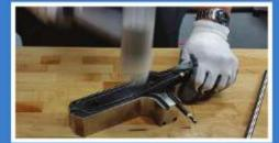
One strong strike is more effective than two soft strikes. If your groove dimensions are correct, you will not damage the internal heater.
