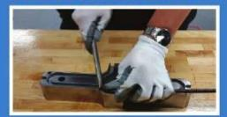
Starting at the center of the groove, use the Nextflex forming tool to bend the Nextflex heater at the center mark consistent with the tool bend.
