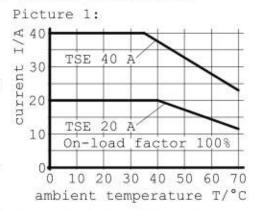
Maximum operating voltage TSE 20 A = 265 V AC, TSE 40 A = 660 V AC. Maximum dissipation loss TSE 20 A = 20 W, TSE 40 A = 40 W.
