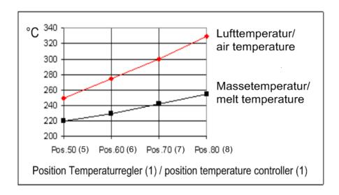
Check temperatures on the running extruder with an external thermometer after about 5 minutes.
