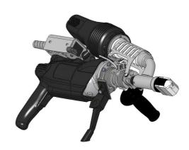
CAUTION Prior to prolonged interruptions of work (approx. 15-30min), set back temperature controller (1) by about 2 positions (risk of overheating of the melt in the melt chamber). Set temperature controller to welding temperature again approx. 5 minutes before resuming work.
