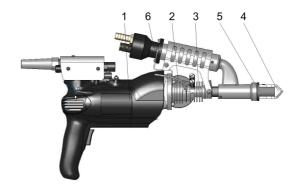
Type **MAK** is a hand extruder with integrated air supply (Autoair).
