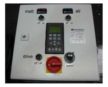
The melt and hot air must have reached the preset start interlock temperatures for the drive to be released by the start interlock. The start interlock temperatures for the melt and hot air temperatures are separately preset.
