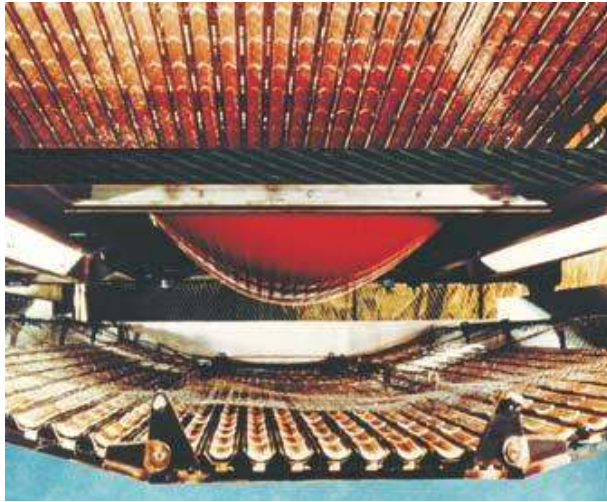
Figure 7: Thermoforming plant for boat hulls
