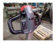
The speed control provides fingertip control for driving the truck
