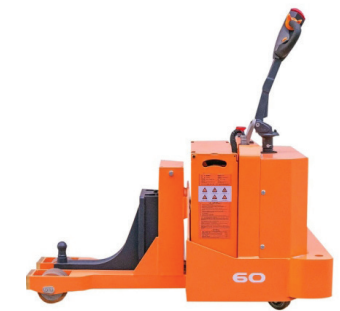
SL XTB 60 Electric Towing Tractor Load capacity 13,000 lbs
