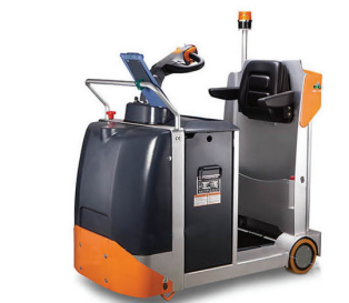
SL XT 30 Operation type Standing on Rate traction capacity 6,600 lbs
