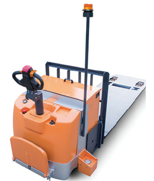
PLATFORM TRUCK Used for moving large size molds and flat glass
