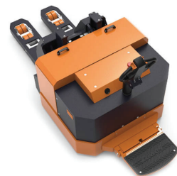
SL XP 100/120 Min fork height 7.9" Load capacity 22,000 / 27,000 lbs
