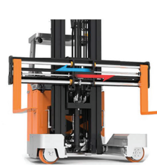
Fork Positioner Max Fork width 98.5"
