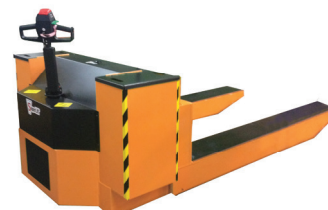
Heavy Duty Forkover Load capacity 25,000 lbs
