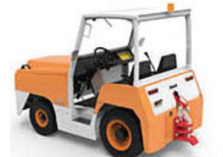
SL XT 250 Operation type Sitting on Rate traction capacity 55,000 lbs
