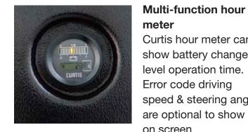
meter Curtis hour meter can show battery change level operation time. Error code driving speed & steering angle are optional to show on screen
