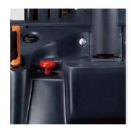
**Emergency stop** switch **Emergency button** will quicky switch off power supply
