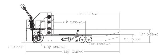
Superlift high performance walk behind pallet truck/fork over capacity to 18,000 lbs with the safety of a pedestrian truck and efficiency of a rider.
