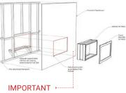
Insulation must be securely wrapped around the firebox body before placing inside opening
