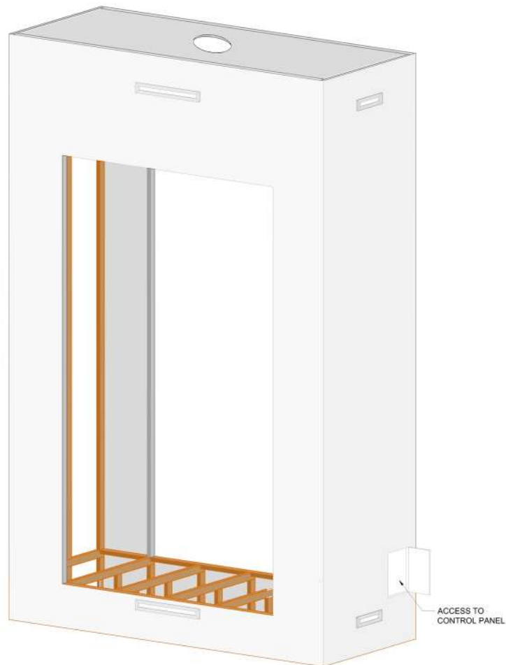
Figure 1.5 (Control panel location)
