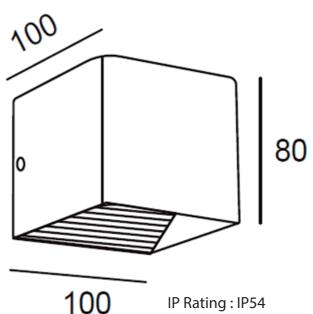
IP Rating: IP54 Colour: 3000K Material: Aluminium Polycarbonate diffuser
