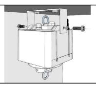
MB A: Bracket to securely mount the lift to the ceiling substrate with two points of fixing.
