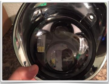
Inspect everything and make sure everything fits snug. Make sure Not to over tighten the screws to the stock plastic housing. I recommend adding a small amount of thread lock to the screws prior to installation. Now plug in the light plug to the bike's wire harness and mount the stock housing back into the stock headlight bucket and Enjoy your New DayMaker. Ride Safe.
