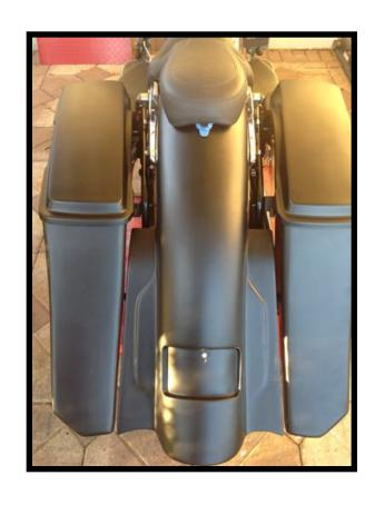
\*\*Once everything is all tighten up and properly mocked up on your new VTX BAGGER it should look like the pictures above. Make sure you have drilled out every hole or notches needed before sending it out to paint\*\*
