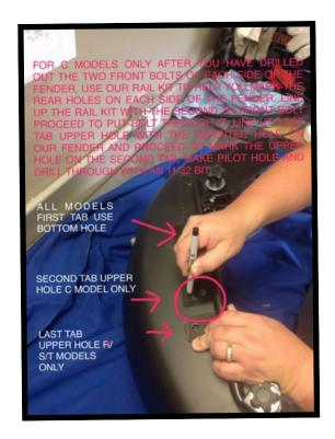
After drilling the final rear hole. You can proceed with the installation of the fender onto your bike, using your stock bolts and lock nuts (not included). If you wish to use your stock fender support bracket continue to next steps.
